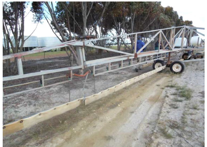
Figure 17. A blanket wiper may be a useful strategy for controlling weeds in French serradella by exploiting height differences between the biserrula and target weed. This model has a very abrasive wiping surface resulting in effective target weed coverage. It also has constant pressure delivery system to the wiping mats which ensures effective delivery.
