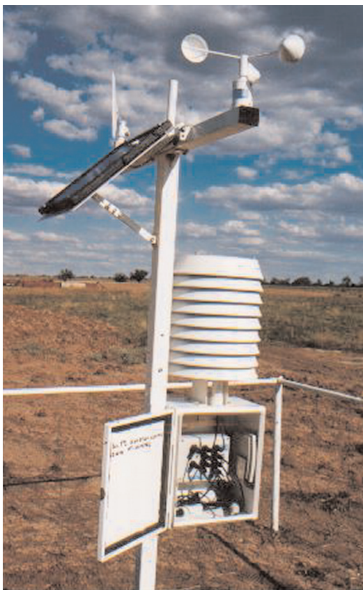
Figure 1: An automatic weather station Photo courtesy of E.A. Systems Pty Limited
