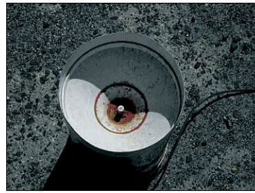
Figure 2: A rainfall sensor clogged with dust Photo courtesy of E.A. Systems Pty Limited
