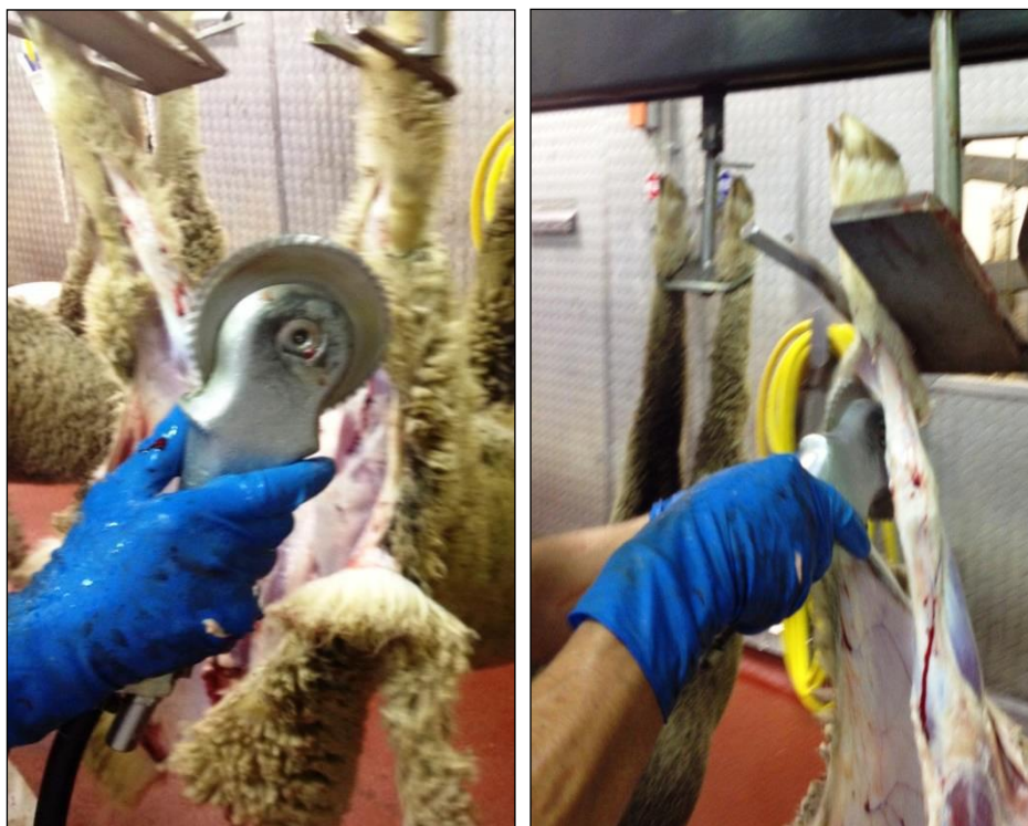
Figure 2: New procedure using air knife.
