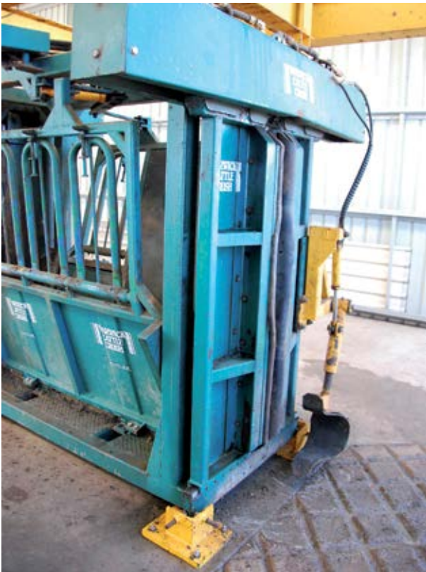
A hydraulically-operated under-chin restraint holds the animal's head steady for more accurate implanting.
